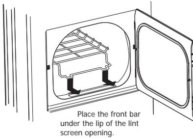
1. Open the dryer door and remove the lint screen.
