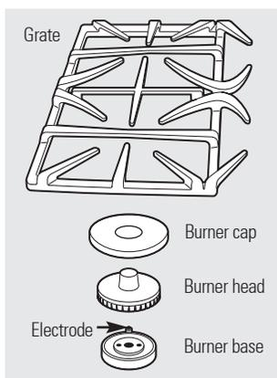
**CAUTION: DO NOT OPERATE THE BURNER WITHOUT ALL BURNER PARTS IN PLACE.**
