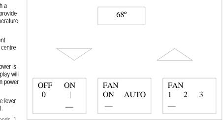
= LOW, 2 = MEDIUM and 3 = HIGH, using the lever switch at the bottom right of the thermostat. To help to create an even temperature throughout your unit, the fan can be run continually at 1 (LOW) speed, providing constant air circulation
