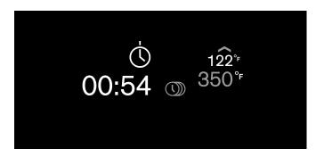
The program will begin with the pre-set warm temperature without light, then advance to the programmed temperature with light until the end of the set date and time, and then maintain the pre-set warm temperature for 60 minutes.
