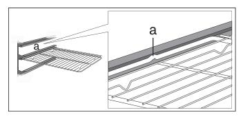
When pushing in the perforated cooking receptacle, make sure that the recess (a) points to the side.
