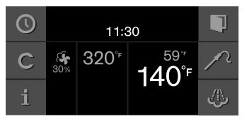
5 The appliance heats with the set heating function. The current core temperature is displayed and, under it, the set core temperature. You can change the set core temperatur at any time.
