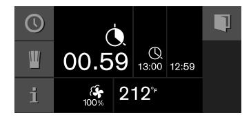
The appliance switches off after expiration of the cooking time. The  $\bigcirc$  pulsates and a signal sounds. It goes off prematurely if you touch the  $\checkmark$  symbol, open the appliance door or set the program selection to  $\bigcirc$ .
