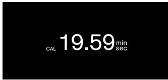
**Note:** Do not interrupt calibration. Do not turn the function selector. Do not open the appliance door.
